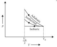
The P-V diagram of an ideal gas compressed from its initial volume  $V_0$  to  $\frac{V_0}{2}$  by several processes is shown in the figure.
